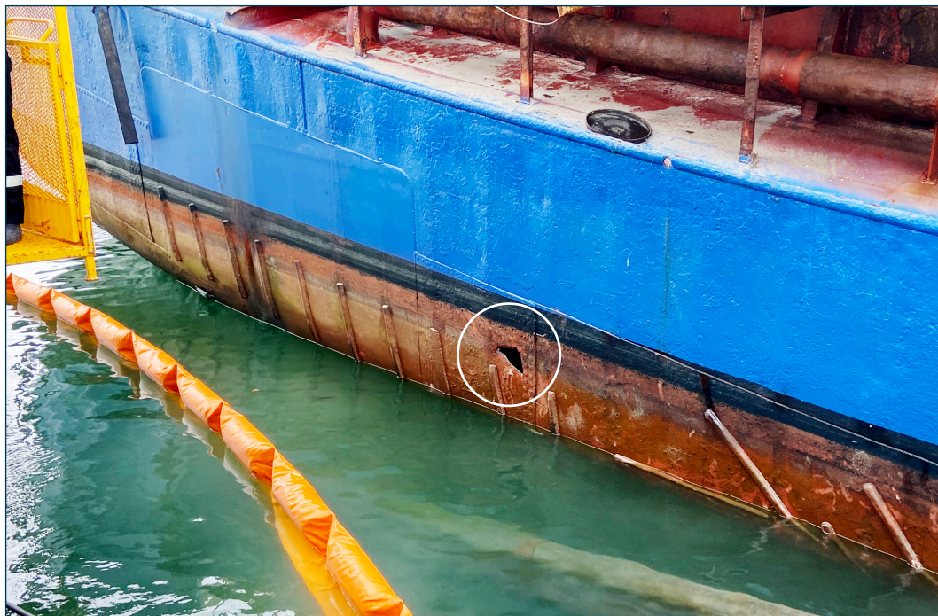
Figur 15: Perforering i klædning, bagbord side. Kilde: Survey Association
